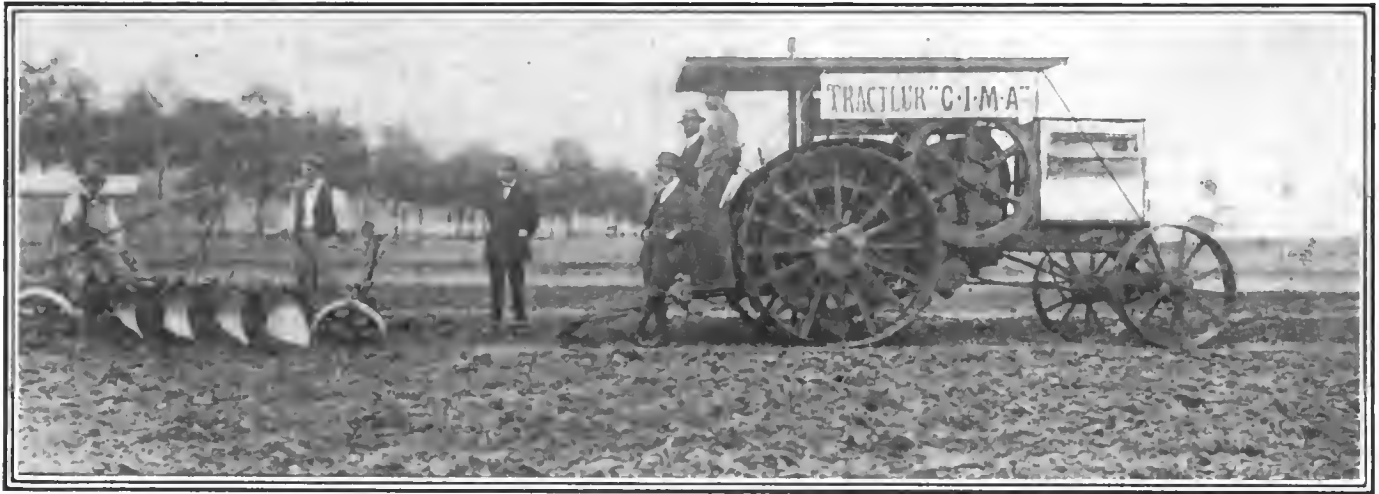
Fig. 1—The C. I. M. A. tractor has a motor with 10-inch bore and 15-inch stroke
